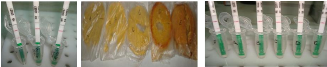
Figure 17. Determination of LOD on GM corn NK603. A) 0.6 %, B) 0.1 % and C) 0.0 %. II. Paste prepared from 0.6 % NK603 sample and baked at: (A) 50 °C, (B) 100 °C, (C) 150 °C, (D) 200 °C and (E) 250 °C.
